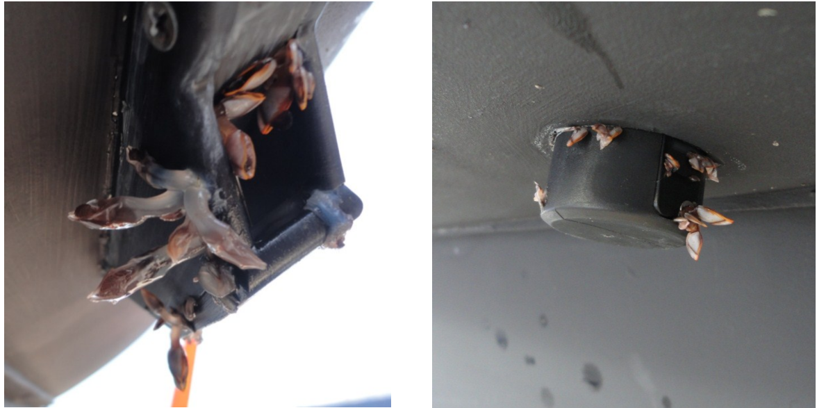
Figure 7. Close-up pictures of the (left) CT-sensor and (right) optode taken after recovery, showing the biology.
