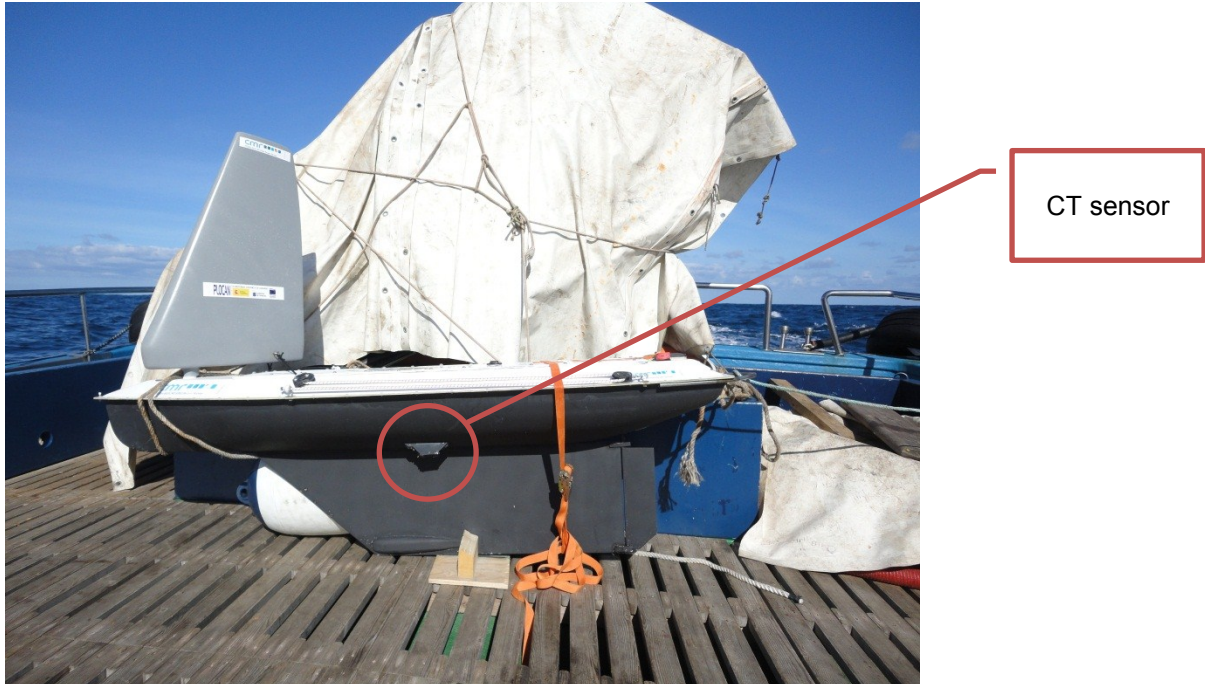
Figure 3. CT sensor mounted on the SailBuoy.
